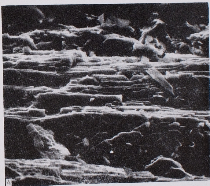
1. Image of secondary electrons (topography) 200 \times 200 \mu\text{m} . Enlarged \times 215 . 2. Mn— K\alpha distribution. Enlarged \times 215 . 3. Si— K\alpha distribution. Electron-probe microanalyse. CAMECA MS-46 \times 215 . 4. Aggregate of plates of investigated Mn silicate. Scanning electron micrograph. Enlarged \times 1000
